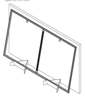
8.1 Screens wider than 400 cm have a top and bottom frame in two frame pieces. Connect the 2 frame pieces with the supplied connection bracket and secure this with the inserted hex screws.
