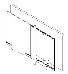
10. First tension the surface so the end of the surface alligns with the frame end. After the entire screen is attached, you can adjust tensioning where necessary.
